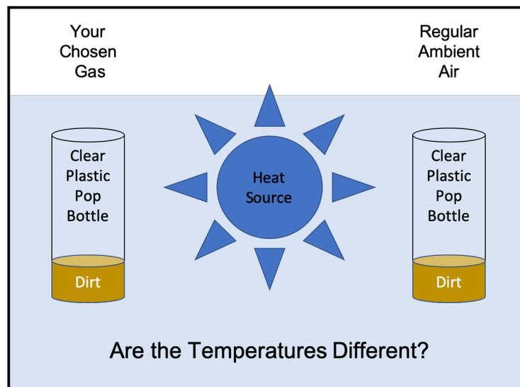
Figure 3: An Easy Experiment to Demonstrate the Greenhouse Gas Effect
