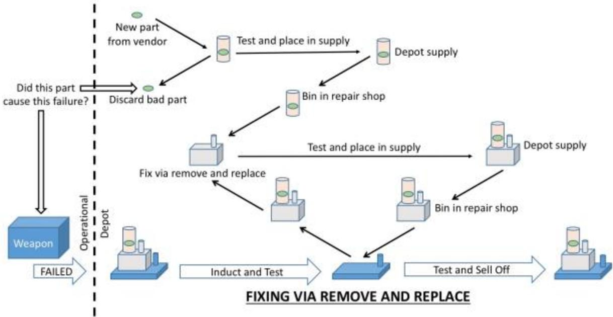
Figure 3: Remove and Replace Depot Repair
